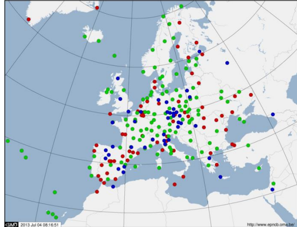
EPN tracking network (status Dec. 2012). Red: stations tracking only GPS signals (31%); Blue: stations tracking GPS+GLONASS signals (51%); Green: stations tracking GPS+GLONASS signals and capable to track Galileo signals (18%).
