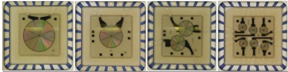
Photographs of the AlN MSM photodiodes mounted on ceramic packaging. The MSM surface area (from left to right) are 4, 3, 2 and 1 mm diameter with 2 \mu\text{m} interdigitated finger width and 5 \mu\text{m} spacing between two electrodes.
