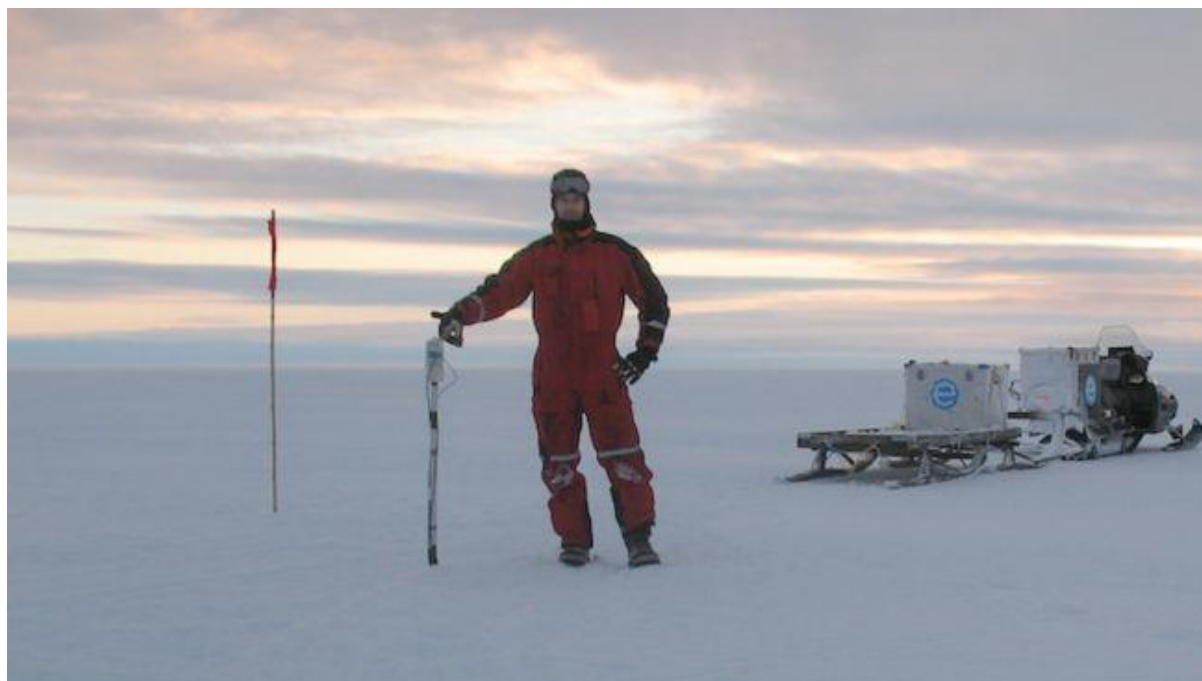
On the Roi Baudouin Ice Shelf, East Antarctica, seismologist Denis Lombardi from the Royal Observatory of Belgium is installing a seismometer (here hidden below the ice) and a GPS device (here visible, mounted on the aluminium pole).
